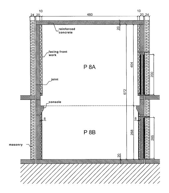
The test facility with suppressed flanking transmission of the testing center accredited according to DIN EN ISO/IEC 17 025 complies with the requirements of standards DIN EN ISO 140, part 1 and DIN EN ISO-140-12. The test facilities allow measurements of various ceiling constructions (e. g. solid slabs, hollow slab floors, hollow filler block floors and single timber floors). A circular console allows the bedding of the individual parts of the ceiling.
