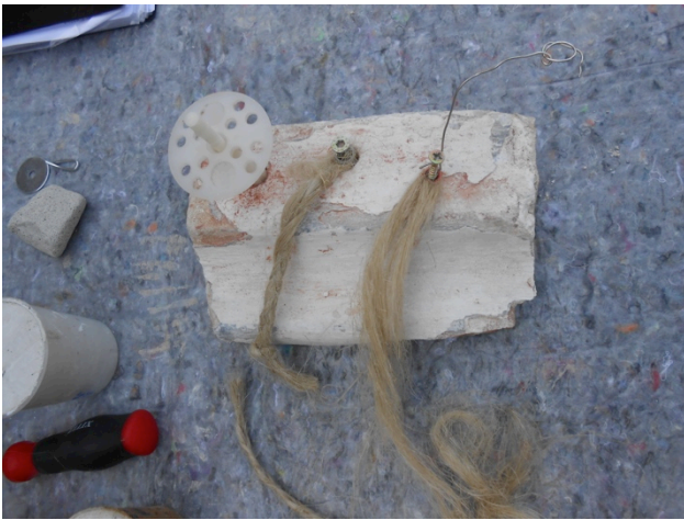
Different ways to secure collapsing fragments using synthetic or natural fibers and various kinds of nails and pins.
