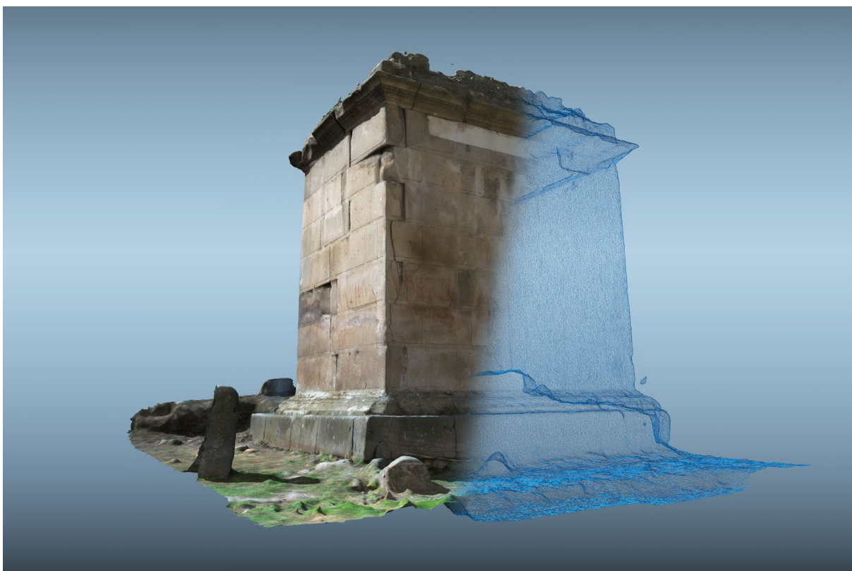
Figure 36. Pompeii. Porta Nocera Necropolis. 17 SO tomb. Texturing the 3D model generated from the point cloud.
