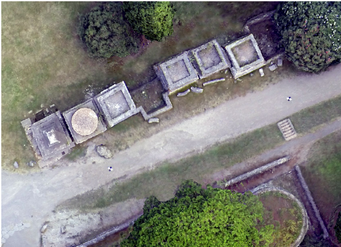
Figure 24. Pompeii. Porta Nocera Necropolis. Ortophotopiano's detail of the investigated area. Visible Ground Control Points for the ground control and georeferencing.
