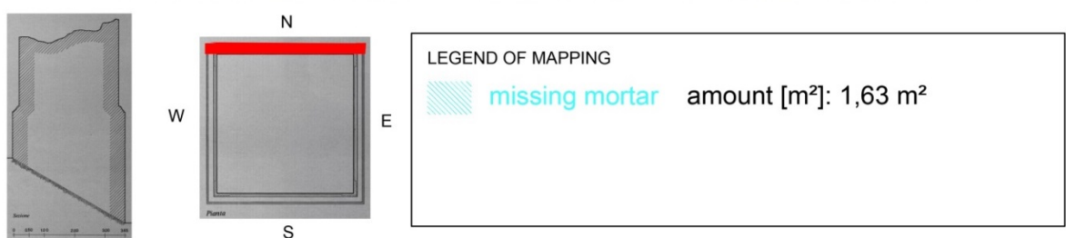
Figure 140: map 14_EN_N of missing mortar.
