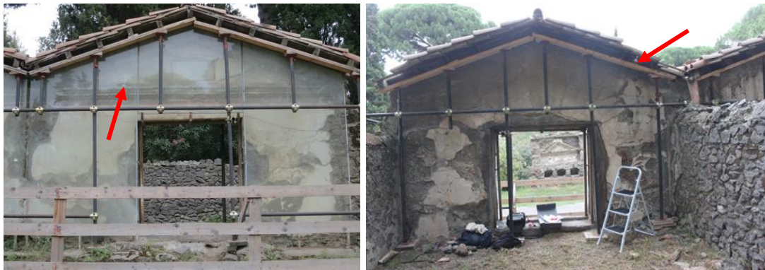
Figure 7: Measurement at tomb ES9 on the front to the street underneath the protective glass. The Sensor is placed on a cornice (red arrow). The right figure shows the rear side of the wall from the inside of the enclosure. The Sensor is placed underneath the wall roof (red arrow).
