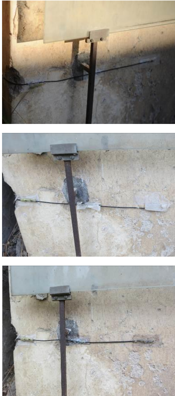
Figure 15: Carefully, reversible mounted sensor on the 2000-year-old original plaster. The upper picture shows the sensor after mounting on 14.11.2014 and the picture in the middle shows the sensor almost falling down on 08.09.2015. Therefore, the sensor was fixed again (lower picture).
