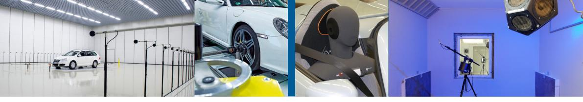
Four-wheel drive chassis dynamometer with semi-anechoic acoustic measuring hall for simulated pass-by mesurements
