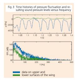
ted in blue and green, respectively. The average of the pressure is smaller on the upper surface than on the lower surface. This difference corresponds to lift. The pressure fluctuation amplitude is larger on the upper surface than on the lower surface. This is because of the turbulent flow generated due to the flow separation above the upper surface. The frequency of the fluctuation is about 25 Hz. The spectrum of the pressure on the upper surface has a broad peak at this frequency.
