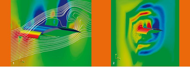
turbulent. Eddies can be observed in the wake. These result in unsteady pressure and give rise to a noise source.
