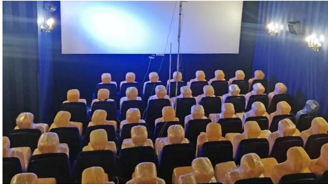
Measurement of the ventilation situation and spread of aerosols in the Neues Rex cinema in Munich. The influence of visitors is simulated by heat load simulators.
